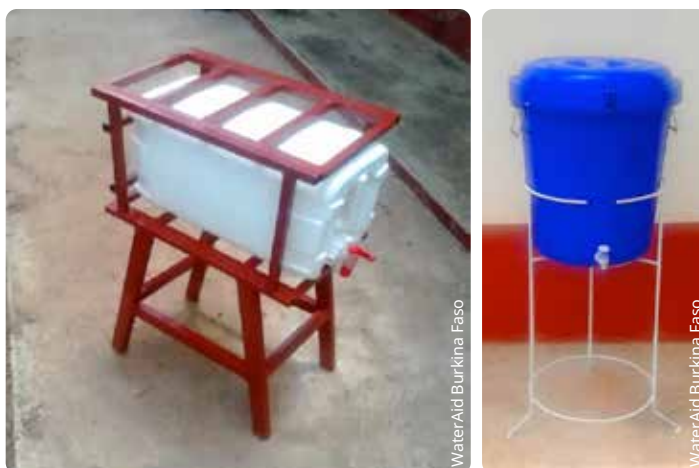
Figure 4: Prototypes of household water storage solutions, tested as part of the research.
