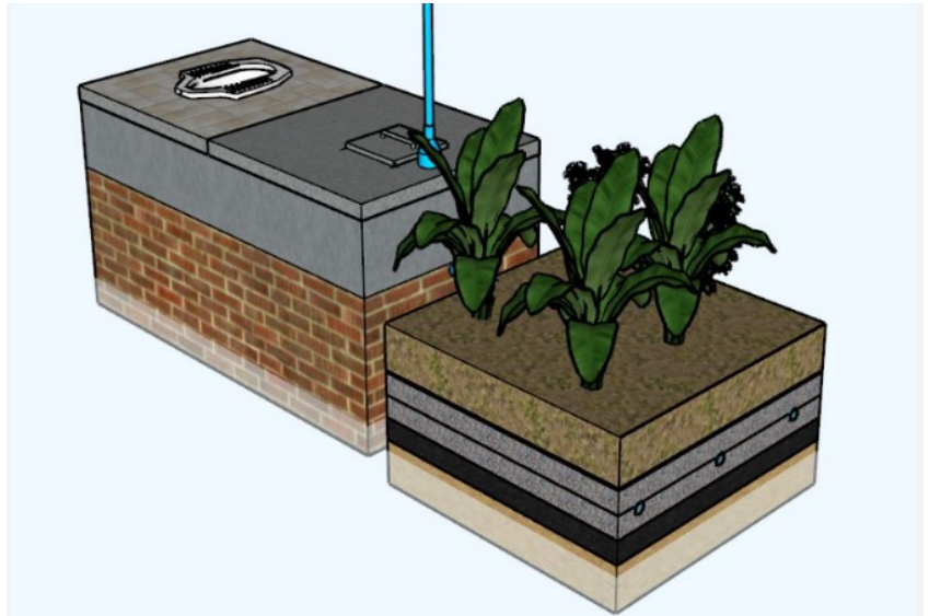
Figure 24. EWB's Septic tank hard ground Sanitation solution
