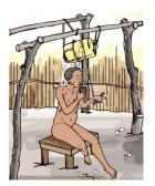
Plastic water container • hung high in bathroom, and tipped forward by • pulling rope so water flows onto bather.
