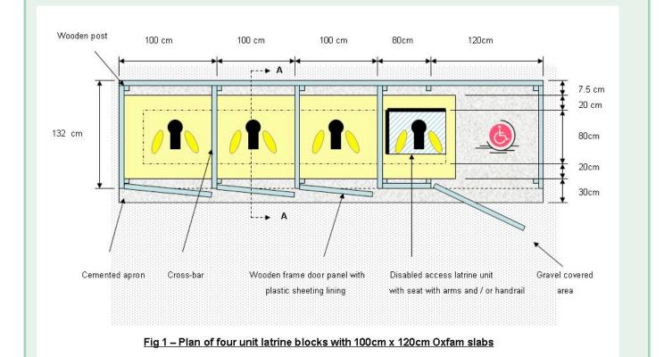
Adding additional space within a latrine unit allows a wheelchair user to enter or a carer to provide assistance. Care is needed to check the sizes and shapes of wheelchairs in the emergency area as this will influence the appropriate sizing of the latrine unit and door.
