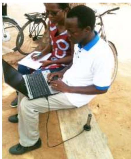
Image 16: Water-level data from a level logger being downloaded to a laptop in the field.
