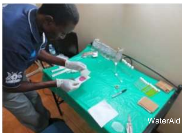
Image 14: Water quality analysis with the Portable Microbiology Laboratory in Uganda, 2015.
