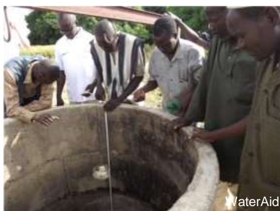
Image 11: Local lecteurs demonstrating a measure of the water level in a well with a whistle device, 2015.
