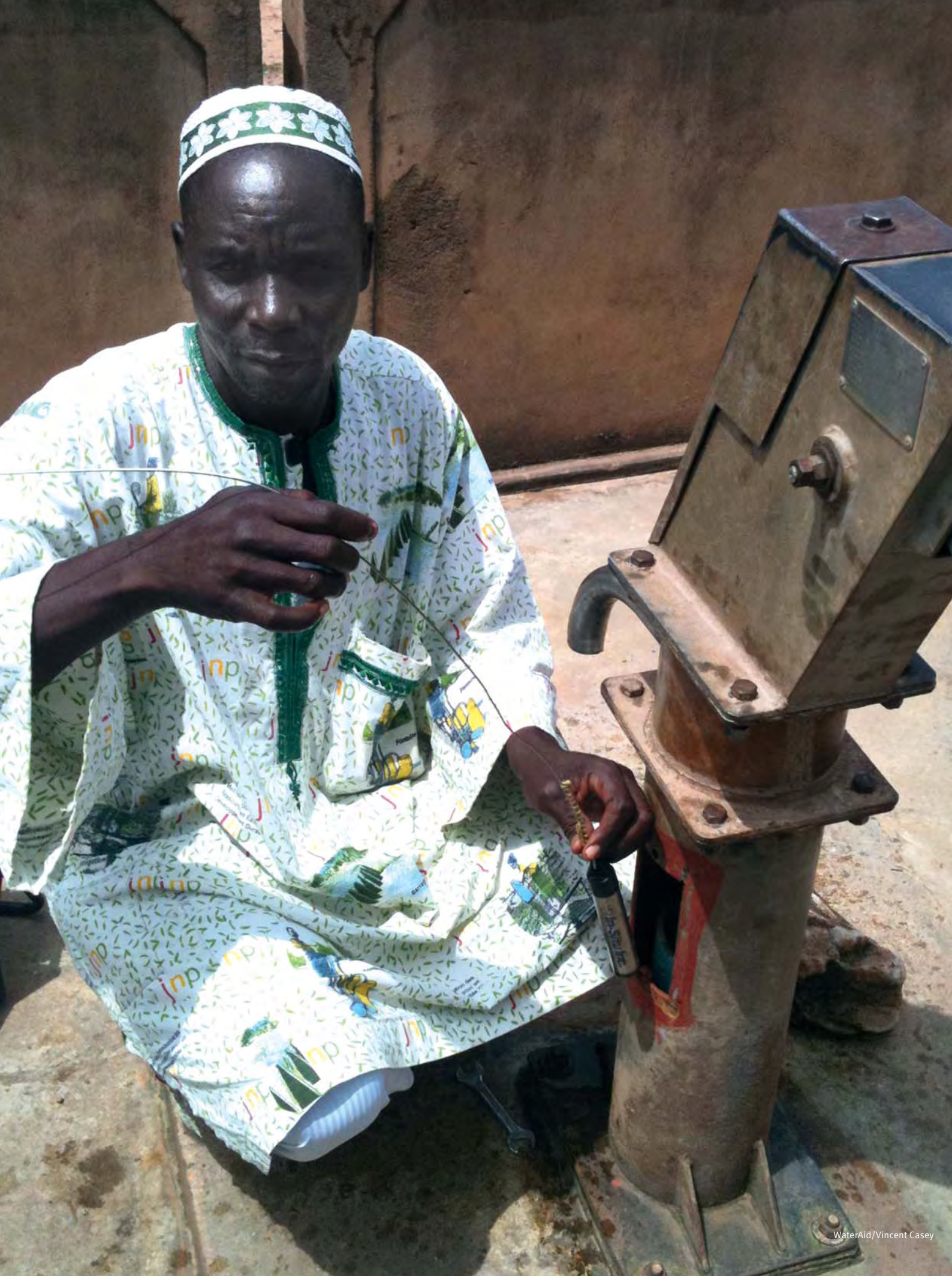
A modified India Mark II handpump pedestal which enables water level readings to be taken in boreholes as part of a CBWRM project in Burkina Faso. Submersible level loggers are being used to record long-term trends in water availability.
