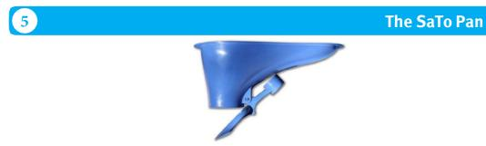
This is the blue plasti cone-cut pan with a flap. It has an attached flipping part that allows passage of faeces and seals up immediately the waste passes into the pit. The SaTo Pan prevents pit heat, smell and flies.
