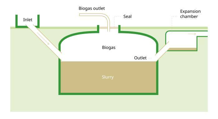
Fig 4: Anaerobic biogas reactor
